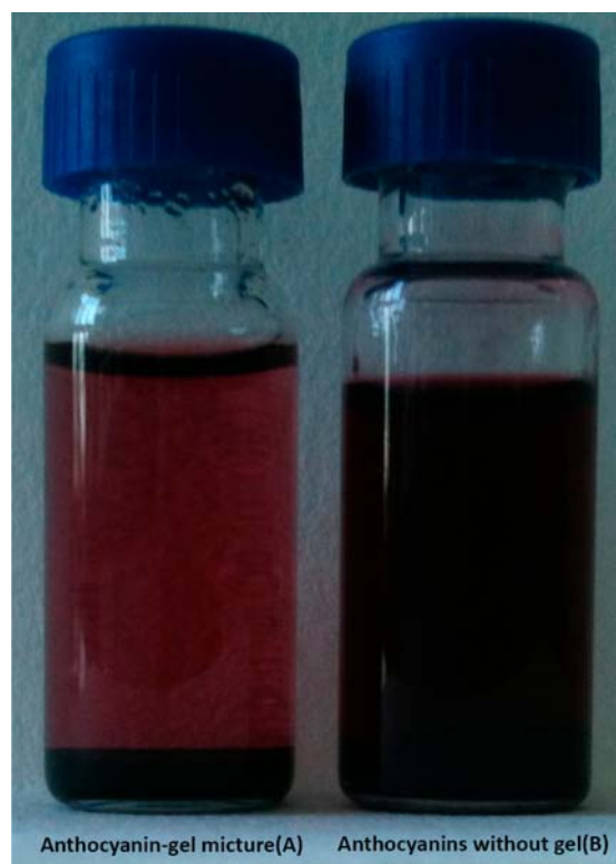
Figure 3. Photograph of anthocyanins–DO100% microgel mixtures (A) and the anthocyanins without gel (B) at pH 3 and ionic strength 0.20 M. The concentration of anthocyanins solution for both cases is around 0.07 mg/mL.
